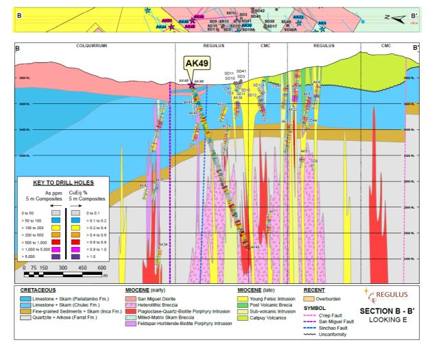
Figure 3 - Cross Section Displaying Hole AK-22-049
