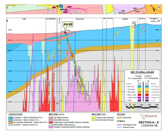
Figure 2 - Cross Section Displaying Hole AK-22-048
