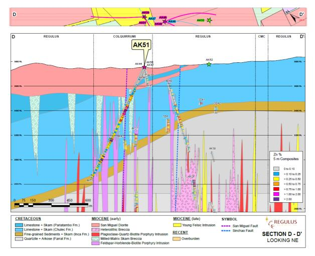
Figure 6 - Cross Section Displaying Hole AK-22-051 (Zinc Only)
